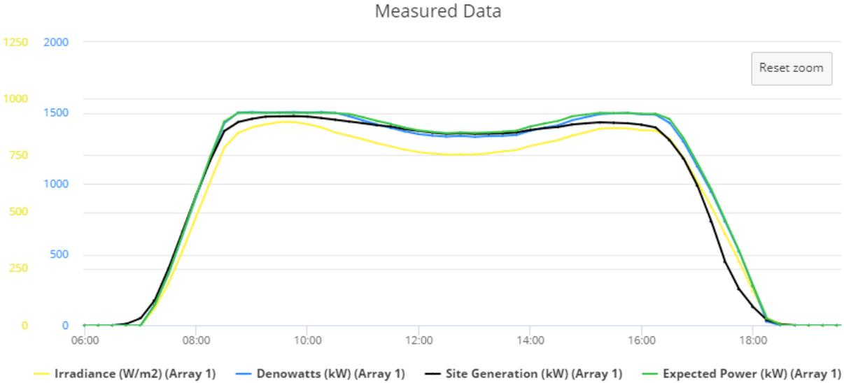
Figure 4: Chart of Expected, Compared, and Generated Power and Irradiance for a Single-Axis Tracker Asset
